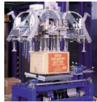
Combination gripper for boxes and pallets
