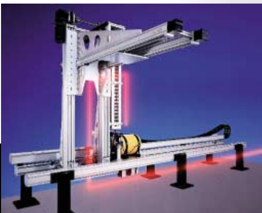
Laser-cleaning of rotor blades
